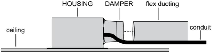
Attach DAMPER to flex ducting with the included DUCT TAPE STRIP.
