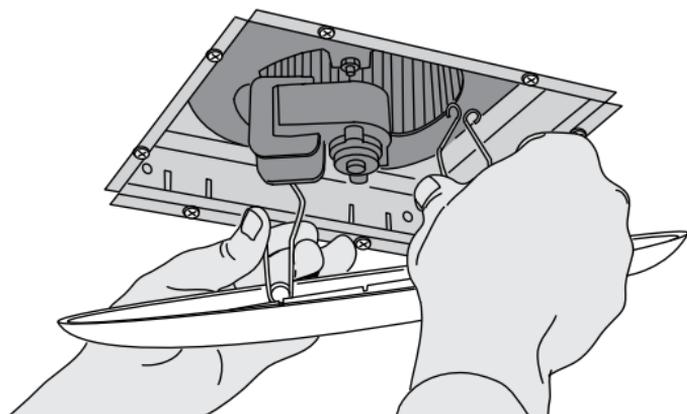
3.) Your existing fan may be attached in several ways. Look for attachment screws in the ceiling and remove. Your fan may also be attached on the attic side and this will require you to access it from the attic. Locate attic attachment screws and remove.
