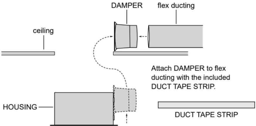
Attach DAMPER to flex ducting with the included DUCT TAPE STRIP.
