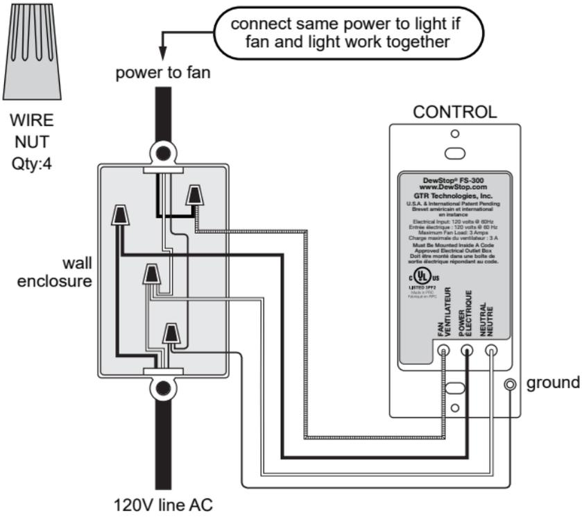
4.) Tuck wires into wall enclosure and fasten the CONTROL to the wall enclosure with the two screws provided.
