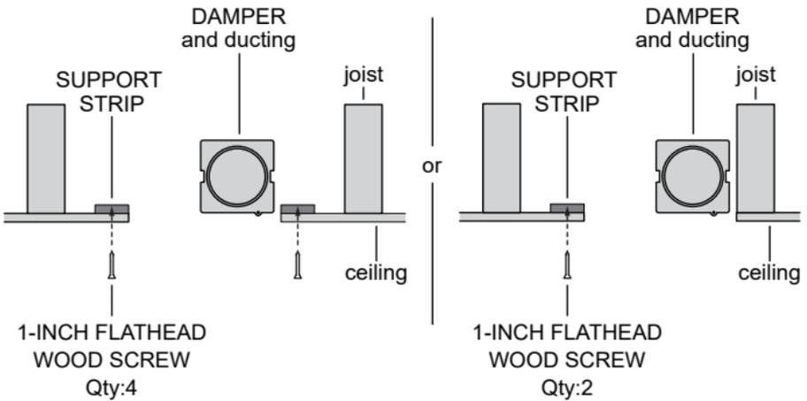
6.) Tilt housing up into ceiling. While tilted, reattach DAMPER through opening in fan HOUSING. Next, use ROUNDHEAD WOOD SCREWS (included) to screw HOUSING into ceiling where you placed the SUPPORT STRIPS.
