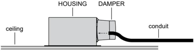
4.) Attach DAMPER to 10.2 cm (4 in) ducting. Use a length of flex ducting, 61 cm (2 ft) maximum.
